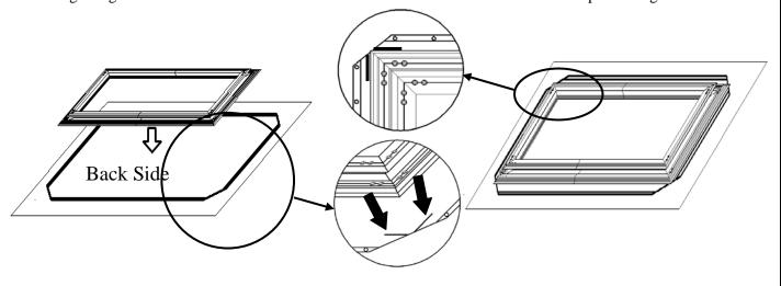
**Step 10:** With one end of the spring and secure inside the groove of the frame, use the *spring hook* (*d*) to attach the spring to the hole located on the screen material's outer edge in the following order.
