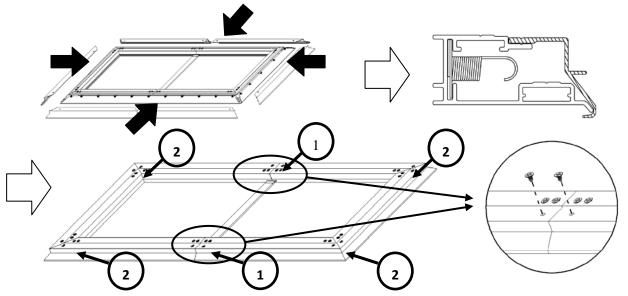
**Step 13**: Install the *angle cover* (j) on each corner of the frame and install the M4x7 screws to hold down the angle cover.
