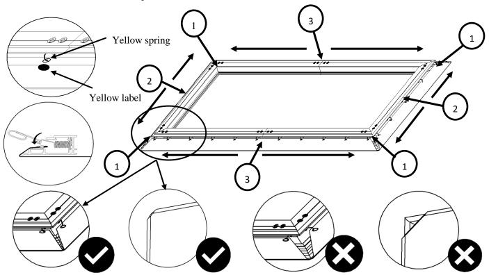
To avoid ripples forming in the material it is imperative that all of the corners are properly wrapped around the edges as illustrated in the check mark diagrams.
