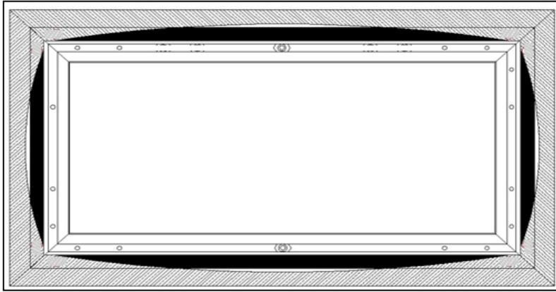
Pull back the screen material from the Velcro connection along the edges of the frame to detach it.
