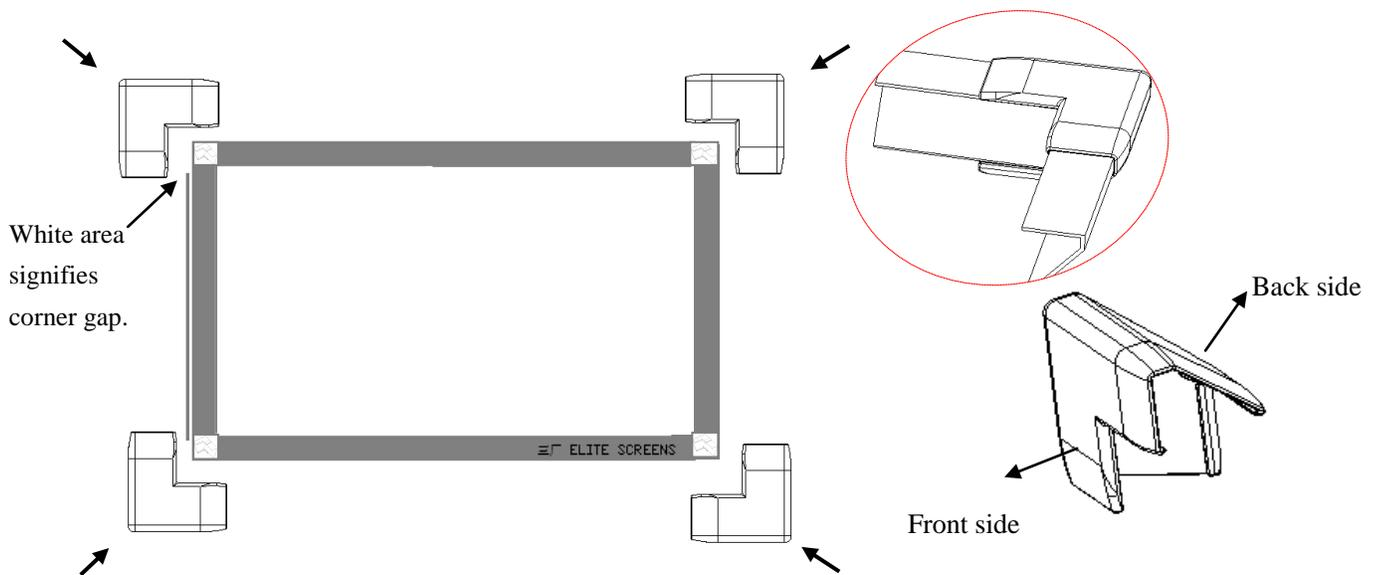
Once all corner sleeves have been snapped into each corner of the frame, it is ready to be wall installation.
