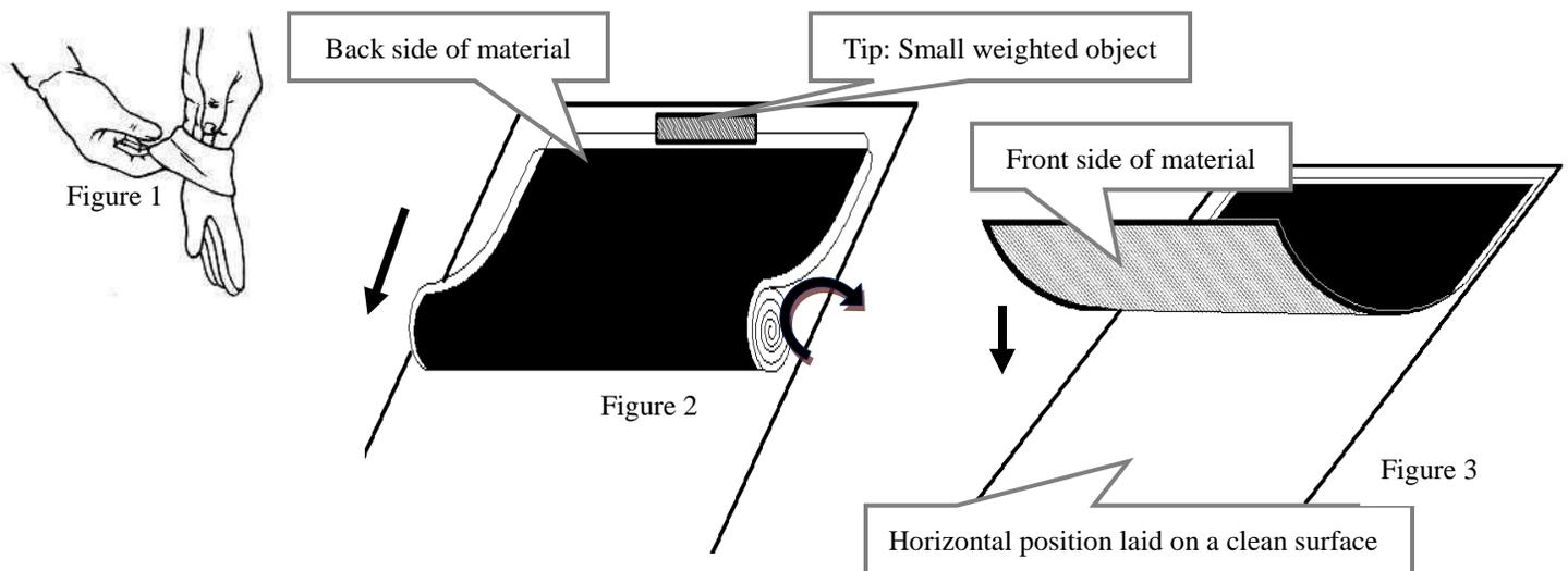
4. Carefully and gently place the assembled frame on top of the screen material as shown below. Make sure to not allow the angle edge of the frame to come in direct contact with the material to avoid puncturing or damaging it.
