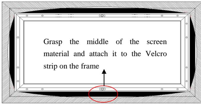
Grasp the middle of the screen material and attach it to the Velcro strip on the frame
