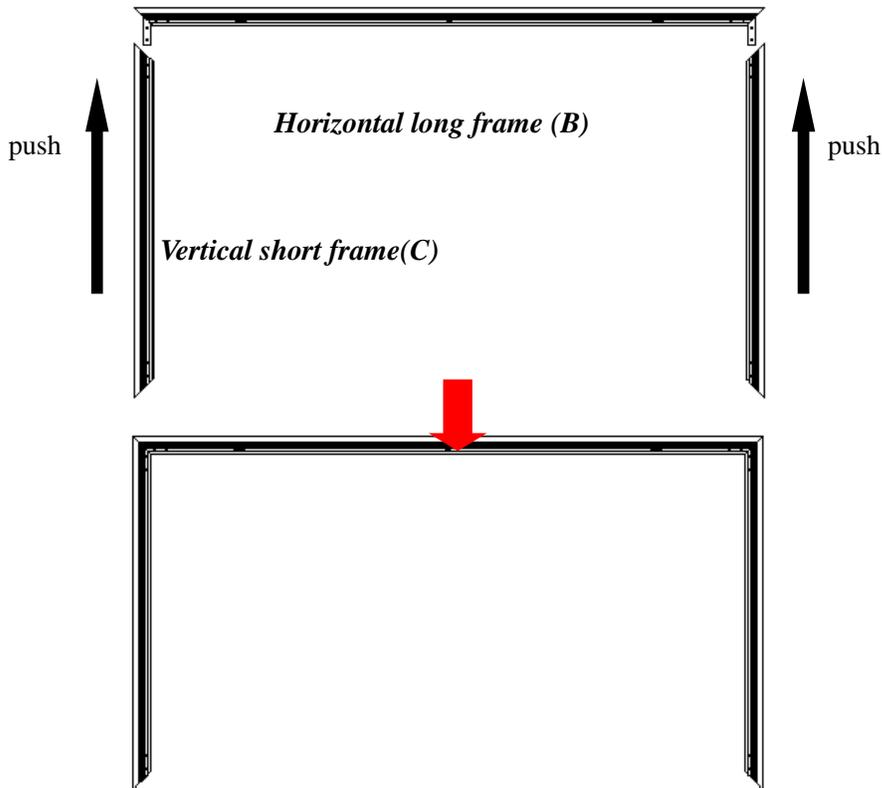
6. Join the remaining *horizontal long frame (B)* with the frame built in the previous steps as shown below.
