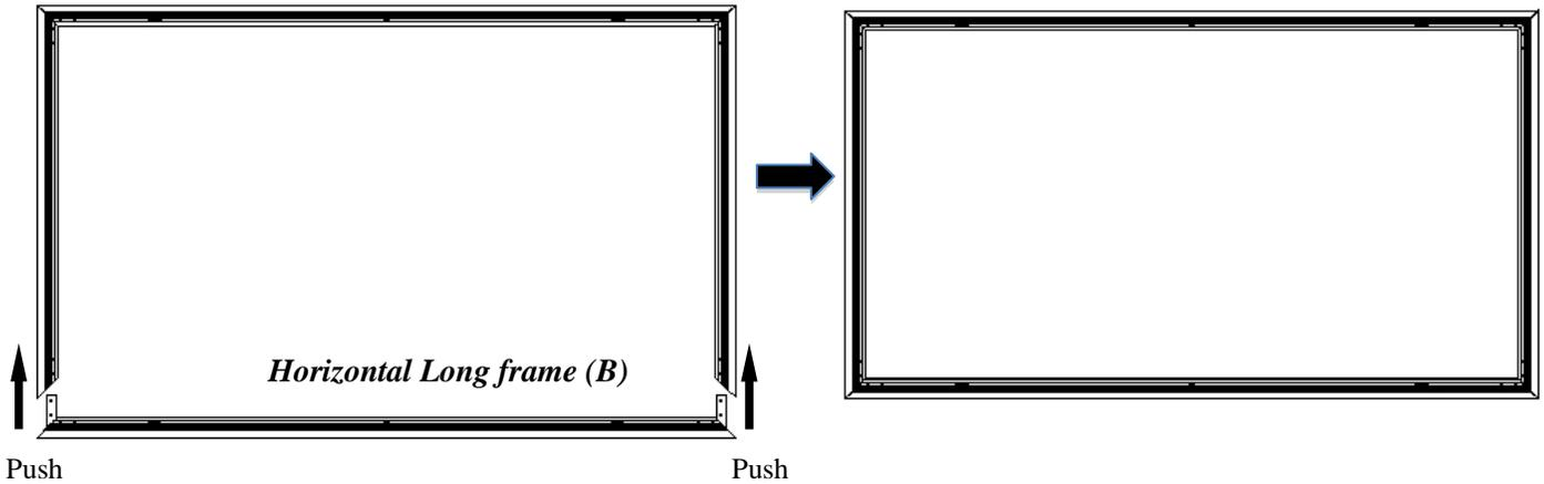
7. Make sure all four corners are properly in place to form a perfect square. Then fasten the four angles with the *M5x15 Screws (G)*.
