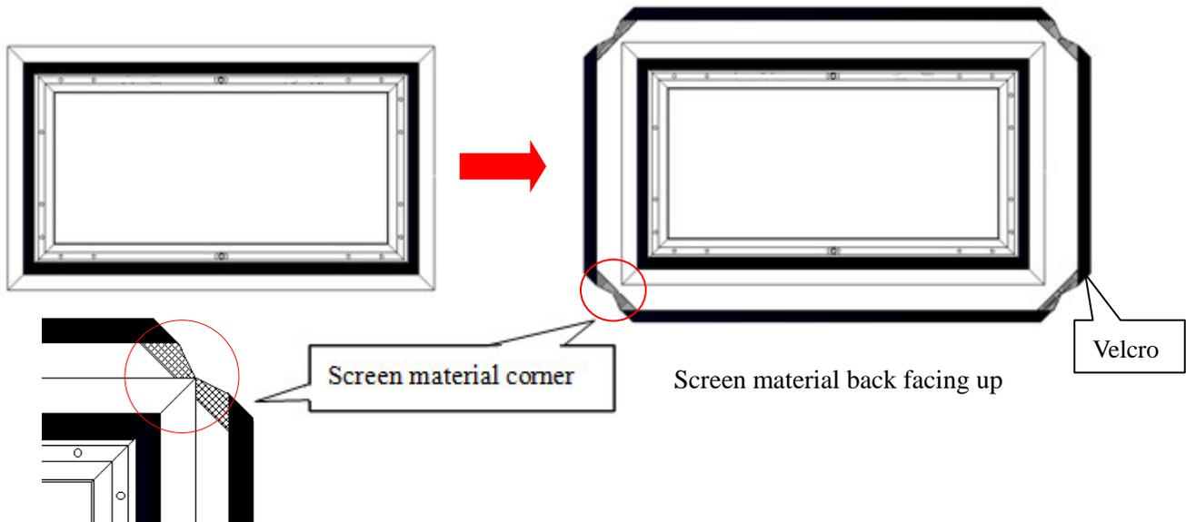
5. After all of the corners of the frame have been properly aligned (example D), attach the material on the frame in the following order A→B→C→D (see instructions below for details).
