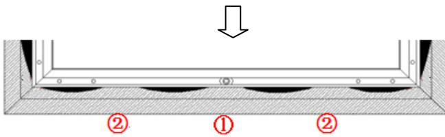
The key is to attach within the middle sections of 1 and 2. Then continue attaching the remaining unattached areas.
