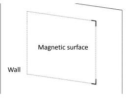
3. Attach the Insta-DEM Screen to the top-right and bottom-right corner of the magnetic surface location as shown below.
