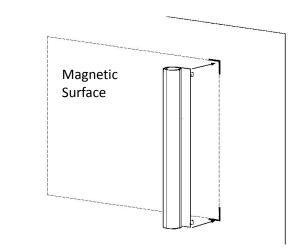
4. Carefully unroll the material and firmly attach the top and bottom until the Insta-DEM Screen is completely attached to the magnetic surface.
