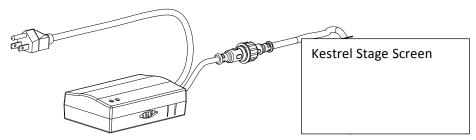
3. After connecting the wall box to the screen, you can operate the screen with the IR, RF remote control or the 3-way wall switch.
